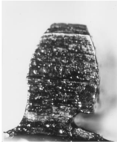
Figure 2. The 33% crack tooth.
